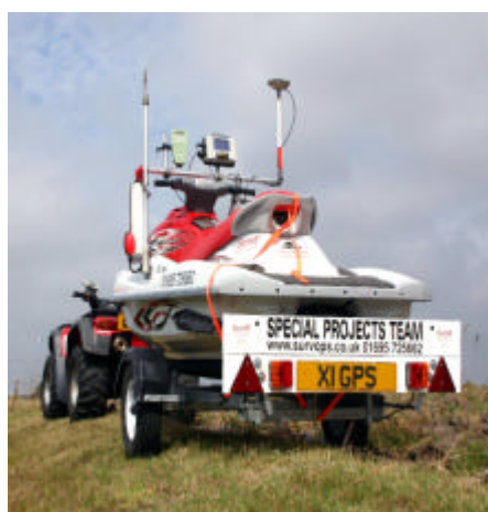
■ Survey Operations Jet Ski fully equipped with Leica GPS1200
